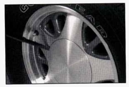
To remove the hub cap from the aluminum wheel, fit the flat end of the extension into the notch.
